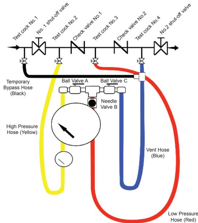
Figure 3 - Reduced Pressure Principle Backflow Preventer
