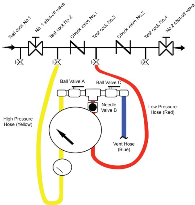
Figure 2 - Reduced Pressure Principle Backflow Preventer
