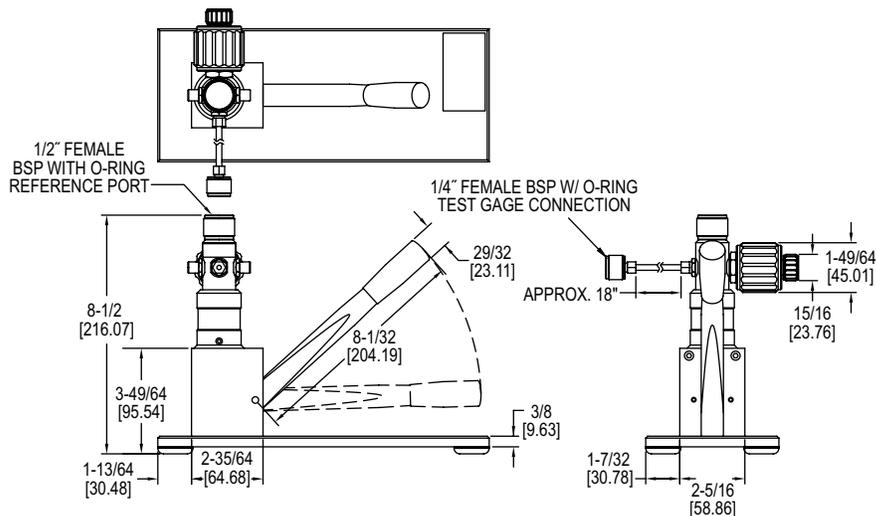
The **Series BCHP Low Pressure Hand Pump** is able to generate pressure and vacuum for adjusting or calibrating pressure gauges, transmitters, or switches. The pump is hand operated and has a pneumatic pressure range of -28 in Hg to 870 psi (-0.95 bar to 60 bar). Dual pressure ports allow two instruments to be connected to the pump without additional fittings. The Series BCHP can be used in laboratories and production areas. The fine adjustment valve on this pump ensures precise measurements.
