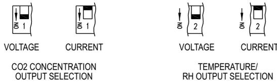
Figure 2: Current/voltage output Selection jumper (PJ1 And PJ2)
