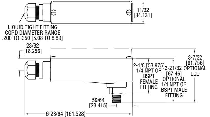
The **Series 626 and 628 Pressure Transmitters** monitors the pressure of compatible gases and liquids with 0.25% full-scale accuracy for 626 models or 1.0% full-scale accuracy for 628 models. The design employs a pressure sensor that can convert a single positive pressure into a standard 4-20 mA output. The Series 626 and 628 are designed to meet NEMA 4X (IP66) construction.
