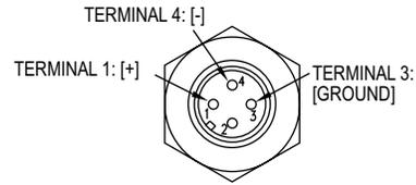
Figure 2: Current output with optional M-12 4 pin connector
