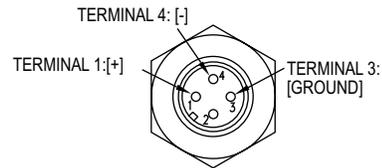
**Figure 3: Current output with optional M-12 4 pin connector**
