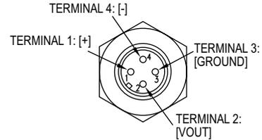
Figure 7: Voltage output with optional M-12 4 pin connector
