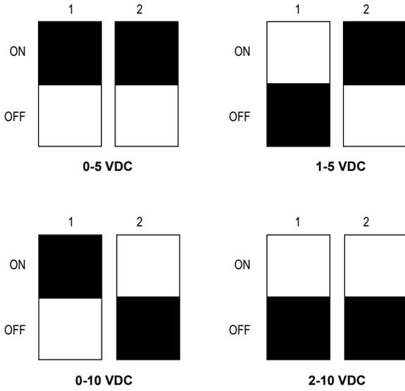
Figure 4: Voltage output DIP switch selection
