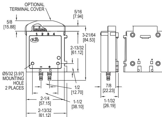
The **Series 616KD One-Touch® Differential Pressure Transmitter** senses the pressure of air and compatible gases and sends a standard 4 to 20 mA or optional voltage output signal. A wide range of models are available factory calibrated to specific ranges. A single push button properly adjusts both zero and span. New enclosure enables the 616KD to be mounted on a 35 mm DIN rail either via its side or back DIN rail clips.
