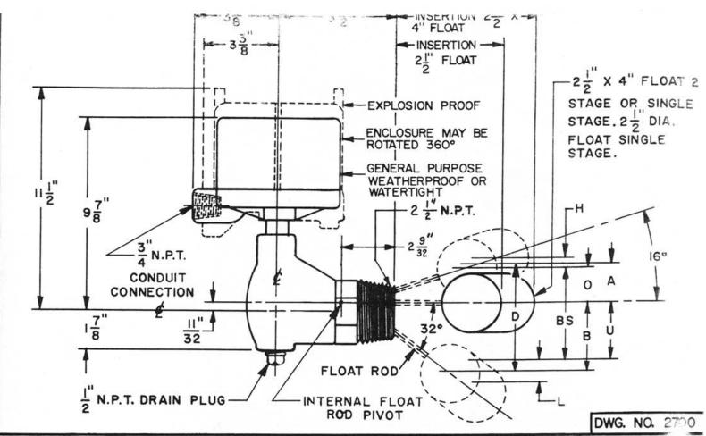
Single Stage(1) Note: Cold shock or water hammer must be avoided, as this condition may damage the float and preven proper operation of the control.
