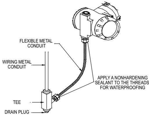
Figure 4-4a: Typical mounting using flexible metal conduit
