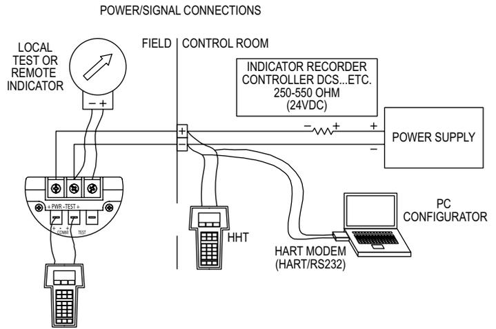
1. HHT (HART COMMUNICATOR) OR PC CONFIGURATOR MAY BE CONNECTED AT ANY TERMINAL POINT IN THE SIGNAL LOOP.
