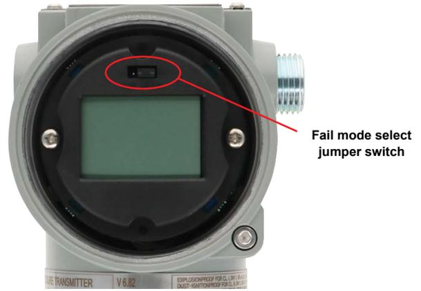
**Figure 3-2: Fail mode selection jumper switch for LCD module**
