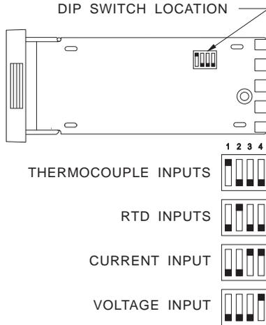
Figure D. Input DIP Switch Location and Settings
