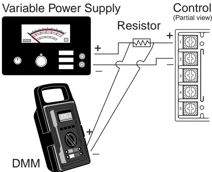
Figure C. Current input wiring.
