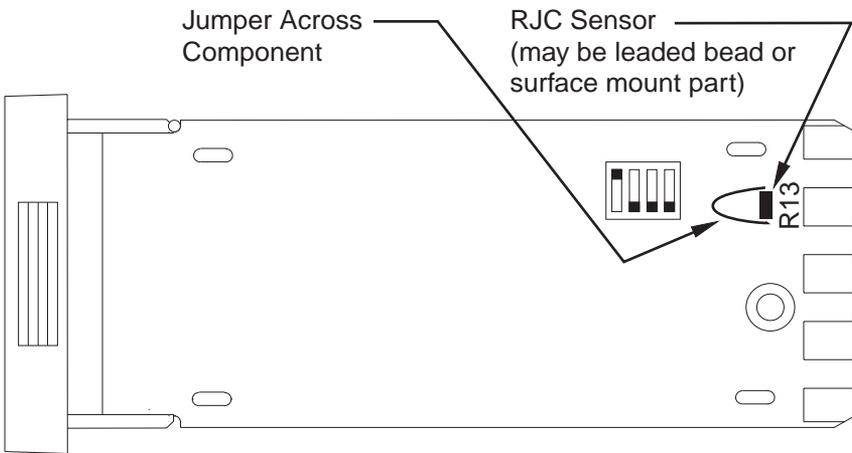
Figure E. RJC sensor and jumper location for 1600 Series
