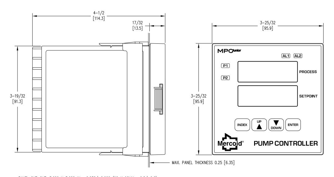
PANEL CUT-OUT: 3.620 X 3.620 IN, +0.032/-0.000 (92 X 92MM, +0.8/-0.0). ALLOW FOR 0.5 IN (13MM) CLEARANCE AT THE REAR OF THE INSTRUMENT.
