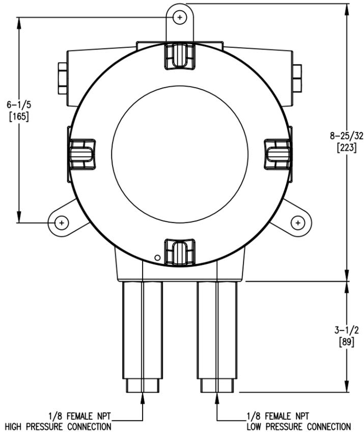
AT-102PA-A3000 (VLO / DTC008 / BACKSIDE VIEW)
